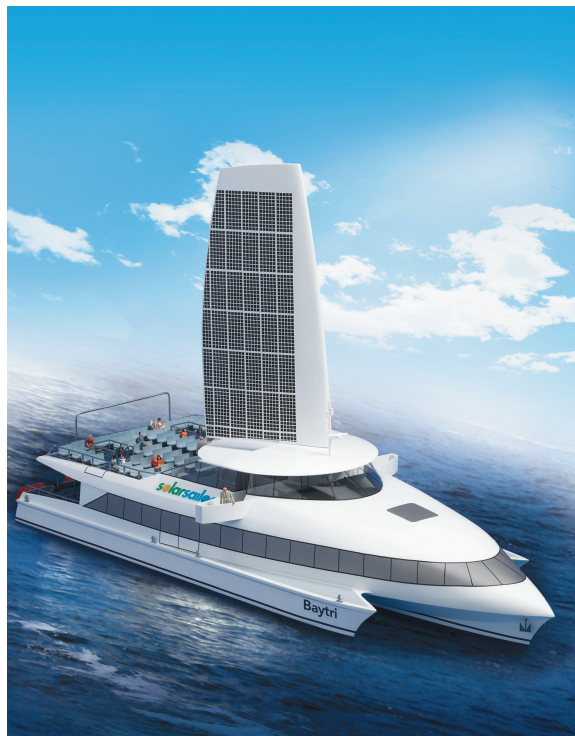
A proposed trimaran for the Alcatraz Island, Calif., run would be solar, electric and diesel powered.
